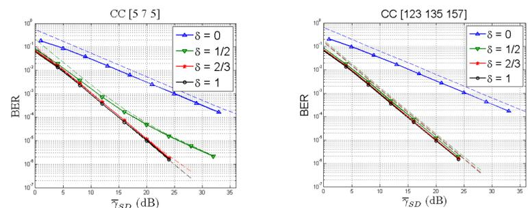
Figure 2: Effect of  $\delta$  on performance of partial relaying for different channel codes. Solid marked curves: simulation results, dotted curves: the upper bound.
