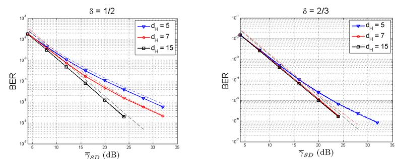
Figure 3: Effect of minimum distance  $d_H$  on performance of the proposed network for different  $\delta$ . Solid marked curves: simulation results, dotted curves: the upper bound.
